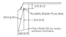
3.2 The dimensions of the **rudder** blade shall conform with the diagram. The **rudder** blade shall be not more than 14mm thick and the thickness shall not vary by more than 1mm to within 25mm of its edges with the exception of hollows or cavities of not more than 2mm in dimension and holes for fixing.
